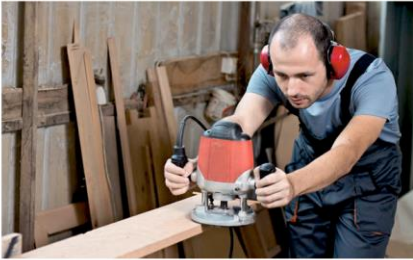
A hand-held router being used to cut a decorative shape into the edge of a piece of timber. The man in the picture above is not following correct health and safety procedures. What is he doing wrong?
