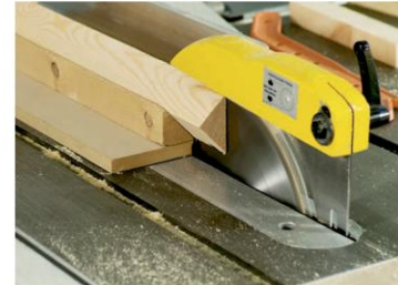
A table circular saw used to cut timber to size: the circular blade makes straight cuts in timber
