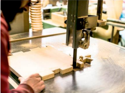
A bandsaw: the blade is one long band with teeth that can make straight and curved cuts in timber. What's wrong in this photo?
