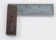
A try square is used to mark a line at 90° to an edge and check if something is square – versatile, may be damaged if dropped
