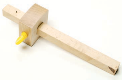
A marking gauge used to mark a line parallel to an edge – can mark out several pieces of timber at the same measurement, the scribing point (spur) scratches the timber so it is vital the gauge is set correctly
